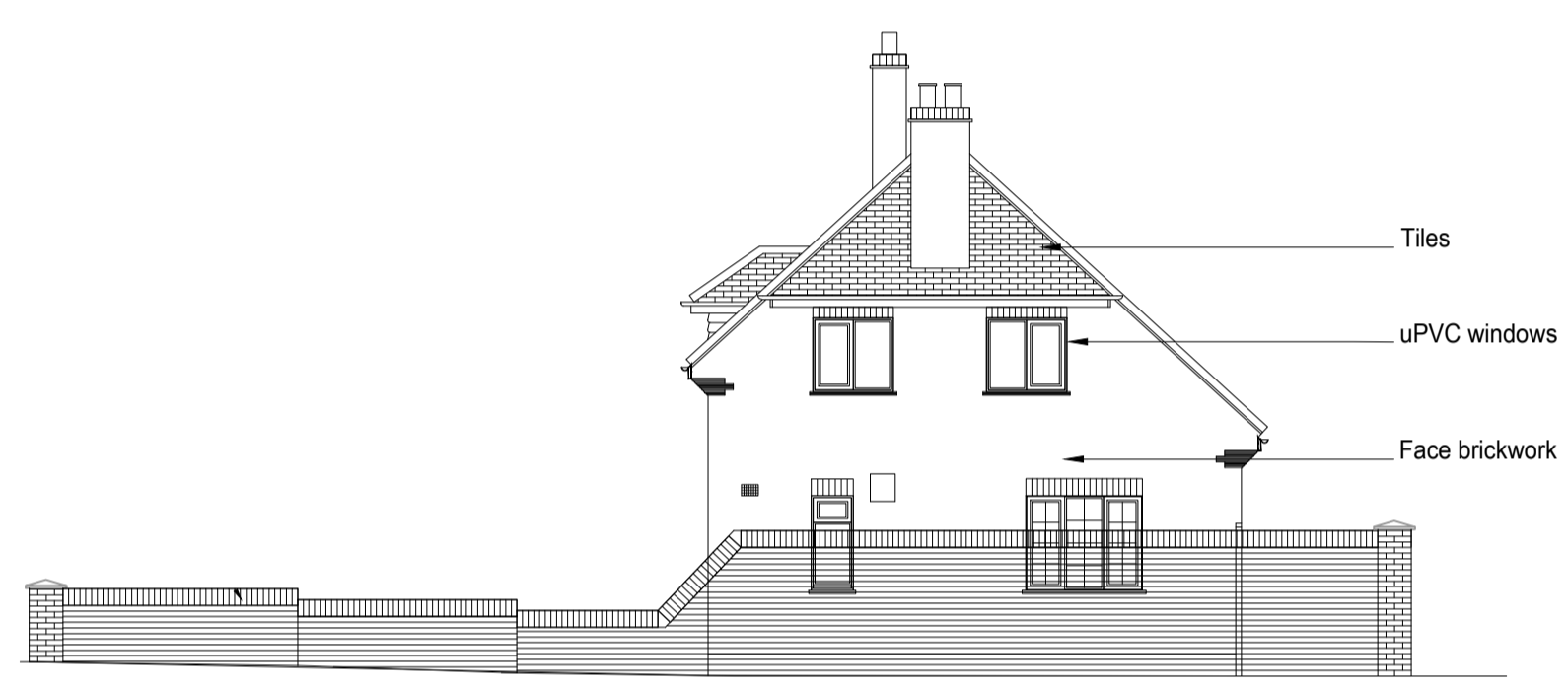
EXISTING SIDE ELEVATION
